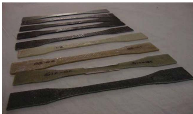
Figure 6 Digital photo of series of G-E composite tensile specimens containing different fillers viz, SiC, Gr, and JOC as per ASTM standard. [Color figure can be viewed in the online issue, which is available at wileyonlinelibrary.com .]
